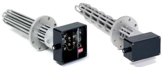
Explosiosproof heating units type GLX for liquids and gases Ex db eb IIC T1-T6 Gb
