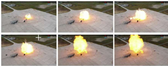
Figure 11: Fireball development after the failure of an MLI-insulated vessel positioned horizontally filled with LH2 as seen from an UAV flying over the H2TA
