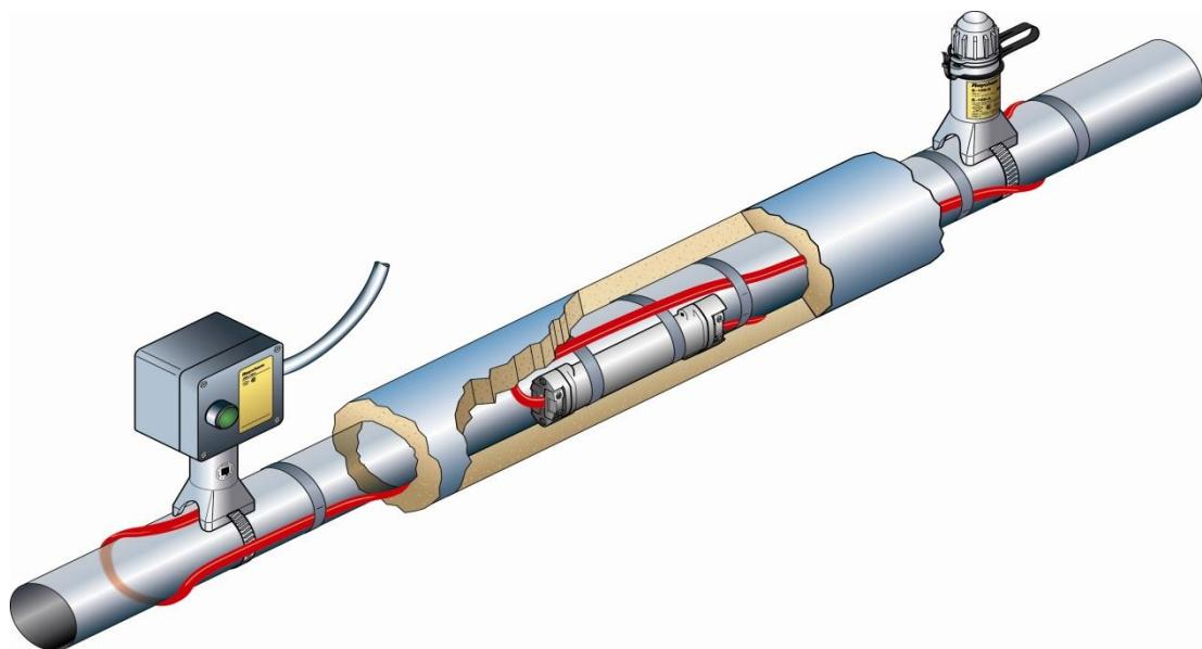
For design, installation and maintenance, the application guide EN 60079-30-2 may be used, this guide is written in conjunction with the product standard EN 60079-30-1, according to which trace heating systems for use in potentially explosive atmospheres are usually assessed and certified.
