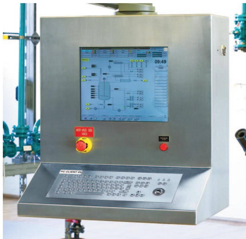
Ex pzc ib [ib Gb] IIC T5 Gc
