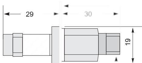
Schlauchanschluss / raccord de tuyau / tube connection
