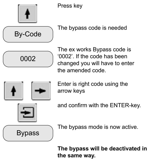
The origin state is normal operation, the Ex p housing can be purged, un-purged or while purging.
