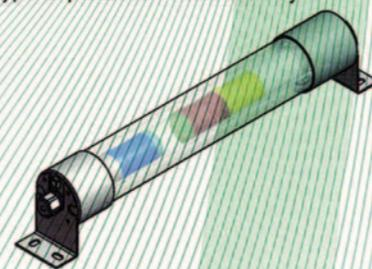
It consists of a transparent tubular housing made from polycarbonate with end caps made of aluminium or stainless steel. One end cap is designed as a blind plug. The other end cap has got either a separately certified cable gland for the fix installed supply line or a separately certified Ex-connector installed for the electrical connection.
