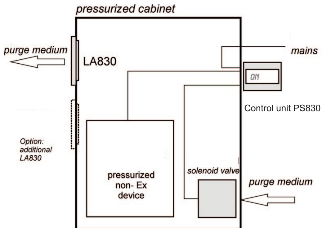
Figure 1 Block diagram
