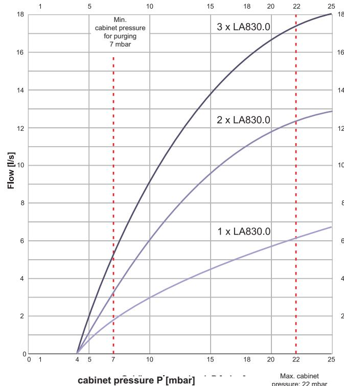
The diagram shows the relationship between pressure inside of enclosure and the output flow. The diagram is only valid, without reducing input or output diameters as well as flow reducing pipes.
